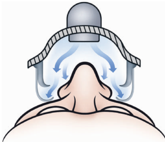
Figure 9.26 Cutaway shows how air pressure flows into the outer cushion of a dual-wall mask interface to enhance the seal, thus reducing the need for excessive head strap tension. (ResMed Mirage system). (© ResMed, 2008. Used with permission.)
